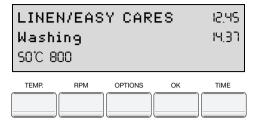
programme adjusts itself to different conditions (e. g., type and quantity of laundry, out of balance spin detection, special rinses, etc.).
